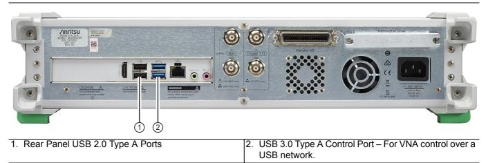
Figure 2-3. Rear Panel Keyboard and Mouse Connections
