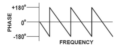
Figure A-16. Linear Phase with Frequency Waveform
